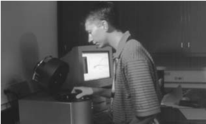
Erik Reisdorf, WSLH advanced microbiologist, loads samples into the LightCycler® real-time PCR instrument. The samples are non-infectious DNA so personal protective equipment is not required in this stage of testing. Photo by Bob Rashid.
