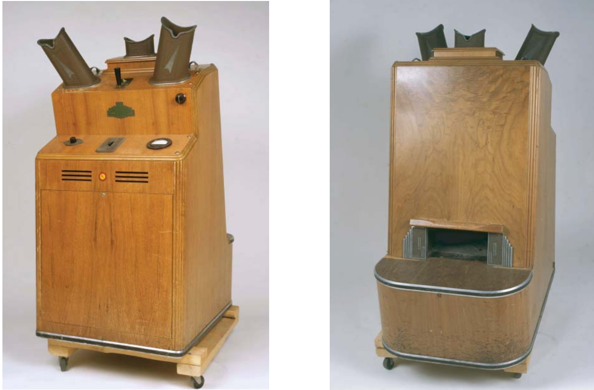
Figure 3. Front and back views of a shoe-fitting fluoroscope. Wisconsin Historical Society, Image IDs: 10419 and 38213.
